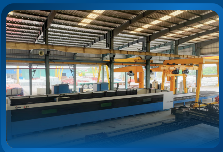
Sheet Metal Fiber Laser Cutting Machines (20 kW, 6 kW & 3 kW)
